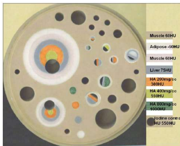
Fig. 1. Custom-made mixed plaque phantom with eight tissue types and ten simulated mixed plaques of various compositions. Contrast agents can be added to the empty holes at desired concentrations. The diameter of the phantom is 100 mm and it can be fit inside a standard QRM thorax phantom.
