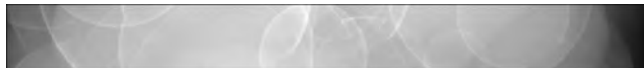
Fig. 2: Example projection from the synthetic dataset with different sized water spheres consisting of 80 overlapped detector rows and 800 channels.
