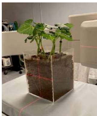
Fig. 1. A sample of a root-soil system imaged to study soil aggregates.
