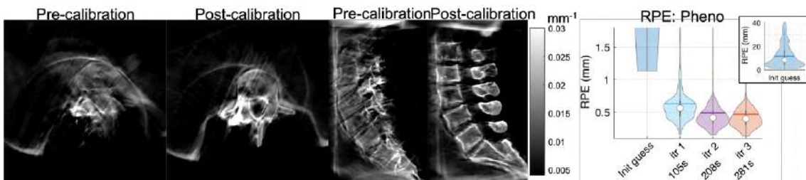
Fig. 7. Experiment C - Artis Pheno: (Left) selected axial and sagittal slices from pre- and post-calibration reconstructions of torso phantom. Voxel size: 0.5 x 0.5 x 0.5 mm. (Right) Summary of RPE as a function of iteration.
